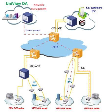
GPN601 works with the packet network and data network. It can manage terminal device by network management VLAN.
